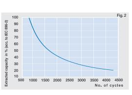
(to Fig. 2) Endurance in cycles according to IEC 896-2 \* S12/85 A = 400 cycles
